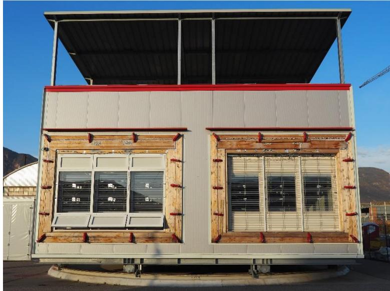
Façade System Interaction Lab - DSF on the left and SSF on the right
